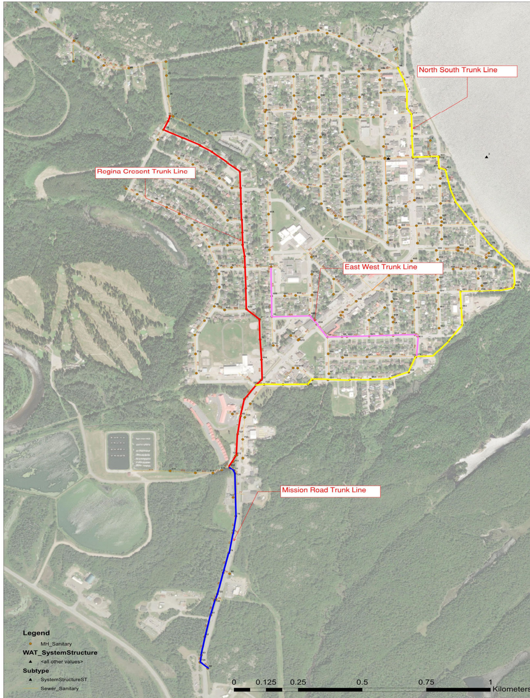
Figure 9: Wastewater Collection System Trunk Lines
